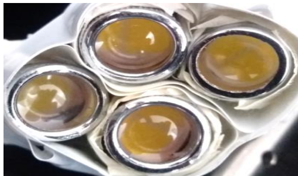
Figure 5. View of the four LEDs, with related optics, used for generating the single light pulse for the ignition tests; LEDs were slightly inclined in order to direct the light to a small area, thus increasing the luminous density.
