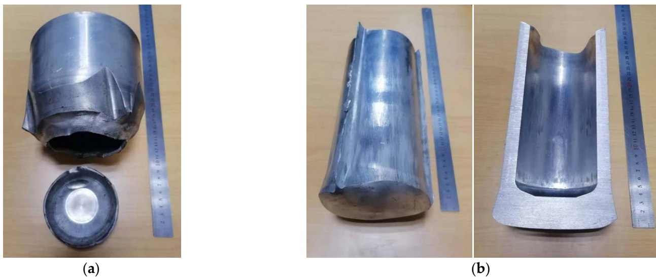
Figure 17. Roll-formed cups: (a) bottom thickness of 20 mm; (b) 30 mm.
