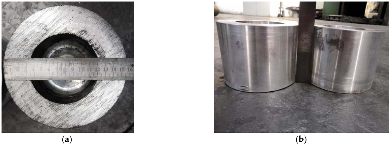
Figure 16. Billets for roll forming: (a) top view; (b) front view.
