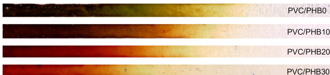
Figure 3. The appearance of the samples after the test for the effectiveness of the residual stabilizer at 220 °C.
