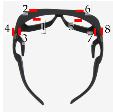
Figure 3. Locations of small dosimeters on radioprotective glasses: 1, left inside lens; 2, left outside lens; 3, left inside frame; 4, left outside frame; 5, right inside lens; 6, right outside lens; 7, right inside frame; and 8, right outside frame.
