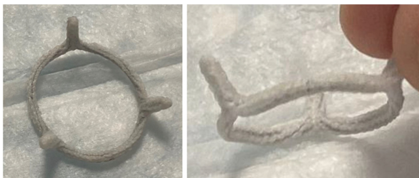
FIGURE 2. A 21-mm ring demonstrating circular deformation with posts flaring outward after dilation with a 24-mm balloon.
