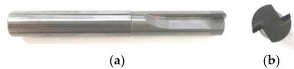
Figure 2. The CVD diamond milling cutter: (a) front view; (b) side view.
