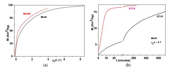
**Figure 4.** (a) Room temperature M–H curves of  $\tau$ -MnAl and  $\tau$ -MnAlC; (b) The M–t plots of  $\varepsilon$ -MnAl during field-heating at 573 K and 673 K, respectively.
