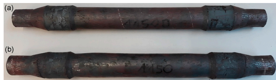
Figure 4. Rail axles rolled: (a) with traditional tools; (b) with multi-wedge tools.
