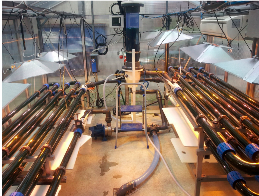
Figure 2. Two-hundred litre tubular photobioreactor with Synechocystis salina CCALA192. The central tower serves as a degasser. The centrifugal pump is situated at the lowest point of the reactor on the left side.
