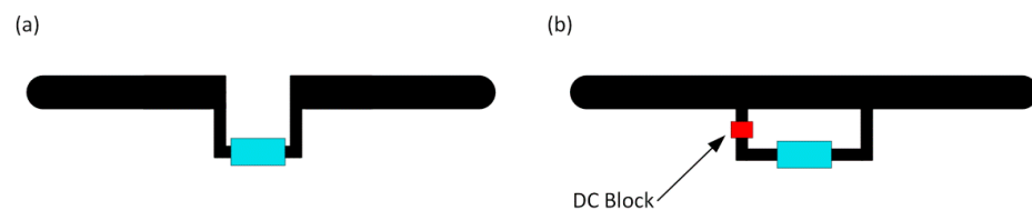
Figure 4. Transponder antenna: (a) Antenna with open arms; (b) Antenna with shorted arms.
