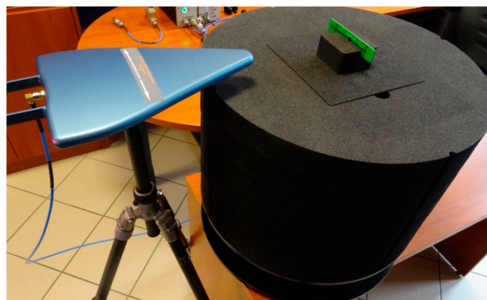
Figure 19. Test stand for radiation pattern determination, in calibration setup.
