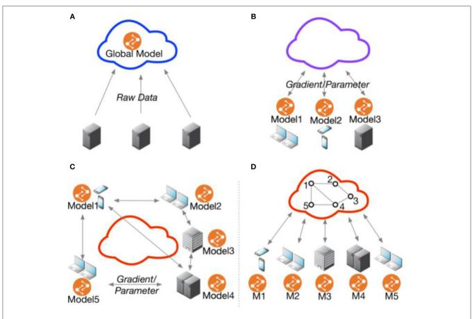
FIGURE 1 | Federated multi-task learning topology. (A) Cloud-based distributed learning; (B) Centralized ederated learning; (C) Decentralized federated learning; (D) Centralized communication topology with decentralized parameter exchanging topology. Adopted from He et al. (48).
