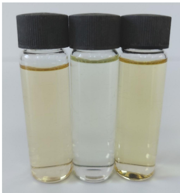
Fig. 3. Color change upon mixing TFQ acceptor ( far left; pale brown ) with the donor ( middle; colorless ) to generate the CT complex ( far right; light brown ). (For interpretation of the references to color in this figure legend, the reader is referred to the web version of this article.)
