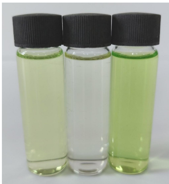
Fig. 4. Color change upon mixing TCNQ acceptor ( far left; light green ) with the donor ( middle; colorless ) to generate the CT complex ( far right; intense green ). (For interpretation of the references to color in this figure legend, the reader is referred to the web version of this article.)
