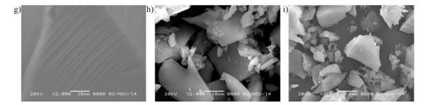
**Figure 6.** SEM images of  $SiO_2$  (**a**,**d**,**g**), VTMSO-SiO<sub>2</sub> (**b**,**e**,**h**), and Q/VTMSO-SiO<sub>2</sub> (**c**,**f**,**i**) with different magnifications.
