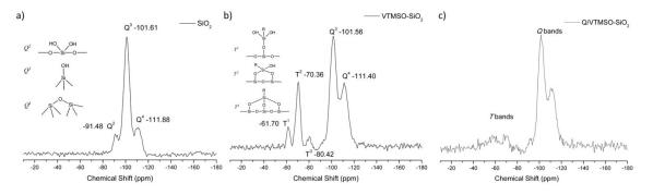
**Figure 1.** Solid-state <sup>29</sup>Si NMR spectra of SiO<sub>2</sub> (**a**), VTMSO-SiO<sub>2</sub> (**b**), and Q/VTMSO-SiO<sub>2</sub> (**c**). Inset: possible structure details with signal assignment.
