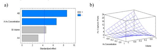
**Figure 8.** (a) Standardized Pareto chart for As capture rate, due to commercial polymer treatment (where: A, As concentration; B, Eluted volume; and AB, AA and BB interactions. Blue line represents critical *t*-value, 95% confidence); and (b) estimated response surface.
