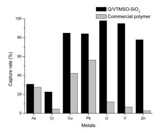
**Figure 10.** Capture rate of some heavy metals present in drinking water by the commercial polymer and Q/VTMSO-SiO<sub>2</sub>.
