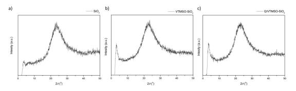
Figure 5. XRD patterns of SiO<sub>2</sub> (a), VTMSO-SiO<sub>2</sub> (b), and Q/VTMSO-SiO<sub>2</sub> (c).
