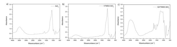
Figure 3. FT-IR spectrum of SiO<sub>2</sub> (a), VTMSO-SiO<sub>2</sub> (b), and Q/VTMSO-SiO<sub>2</sub> (c).
