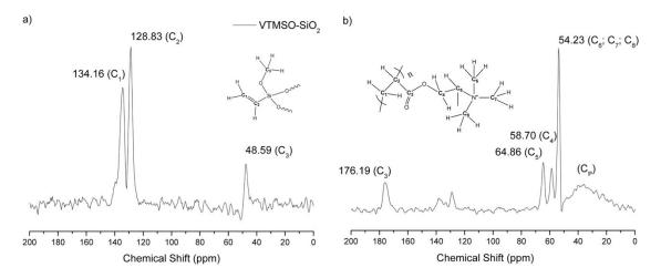
**Figure 2.** Solid-state <sup>13</sup>C NMR spectrum of VTMSO-SiO<sub>2</sub> (**a**) and Q/VTMSO-SiO<sub>2</sub> (**b**). Inset: structure details with signal assignment.
