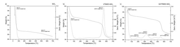
Figure 4. TG-DTG thermograms of SiO<sub>2</sub> (a), VTMSO-SiO<sub>2</sub> (b), and Q/VTMSO-SiO<sub>2</sub> (c).
