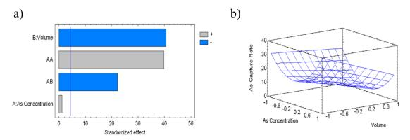
**Figure 9.** (a) Standardized Pareto chart for As capture rate, due to Q/VTMSO-SiO<sub>2</sub> filler treatment (where: A, As concentration; B, Eluted volume; and AB, AA and BB interactions. Blue line represents critical *t*-value, 95% confidence); and (b) estimated response surface.
