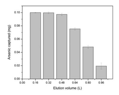
**Figure 7.** Affinity assays between Q/VTMSO-SiO<sub>2</sub> and arsenic solution (0.1 mg $\cdot$ L<sup>-1</sup>).
