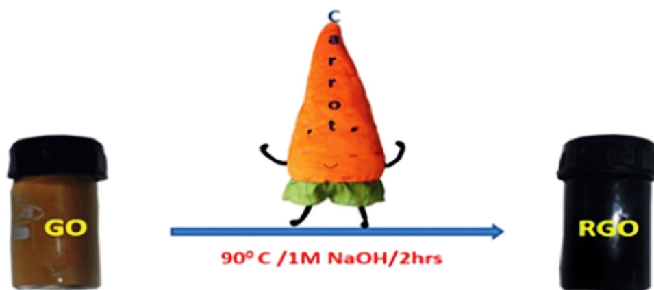
Fig. 4 Schematic representing the reduction of GO by carrot. (Reproduced with permission from RSC Advances 4, no. 43 (May 23, 2014): 22,470–75, https://doi.org/10.1039/C4RA01718H .)
