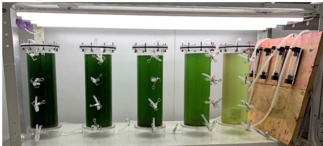
Figure 1. PSBR with Consortia with algae/sludge 10:1, 5:1, 1:1, 1:5 and 1:10 (donated as R1 to R5).
