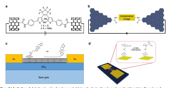
Figure 3 | Applications of photochromic carbon-based nanomaterials in molecular junctions (upper images) and transistors (lower images). Amide formation is used (a) to bridge two CNTs with a diarylethene molecule. Adapted from ref. 82 (Copyright 2007 American Chemical Society) and
