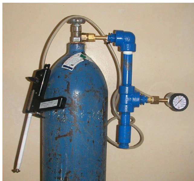
Figure 2 A picture of the cryotherapy gas conditioner with an Ascon Cryosurgery device.
