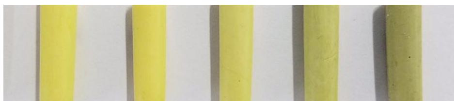
Figure 4. Appearances of polyimide (PI) aerogels with different A-AgNWs contents. From left to right PI-0, PI-0.1, PI-0.2, PI-0.5, PI-2.
