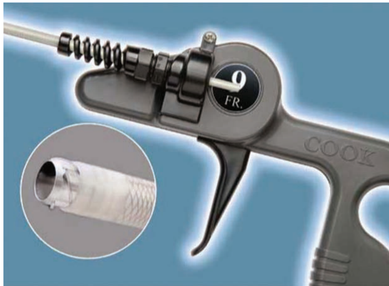
Figure 10: The Evolution ® and Evolution ® Shortie Mechanical Dilator Sheaths (Cook Medical, Bloomington, IN, USA). These “hand-powered” mechanical sheaths consist of a flexible, braided stainless steel sheath with a stainless steel spiral-cut dissection tip (inset). The sheath is attached to a trigger handle that rotates the sheath and allows for the threaded metal end to auger out the scar tissue. Courtesy of Cook Medical, Inc.
