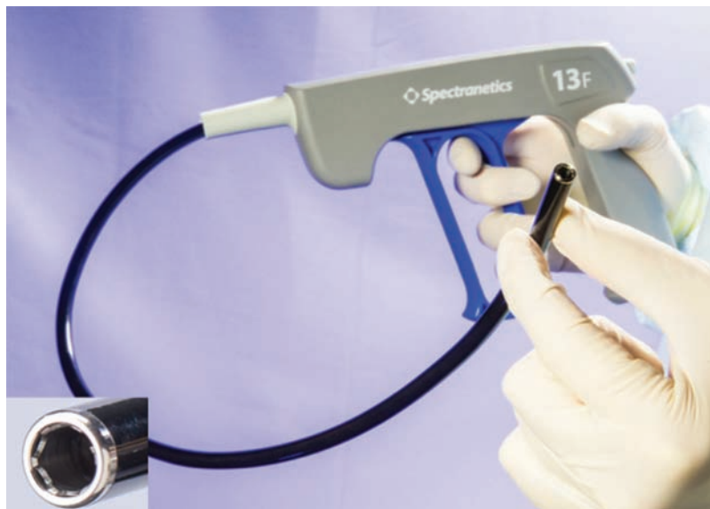
Figure 9: The TightRail™ Mechanical Dilator Sheaths (Spectranetics, Colorado Springs, CO, USA). The flexible shaft, shielded bidirectional rotating blade and static sheath are unique features that allow for the device to pass through dense and calcific scarring while requiring less traction force. The inset image is a magnified view of the sheath tip with the shielded metal blade. Courtesy of the The Spectranetics Corporation.
