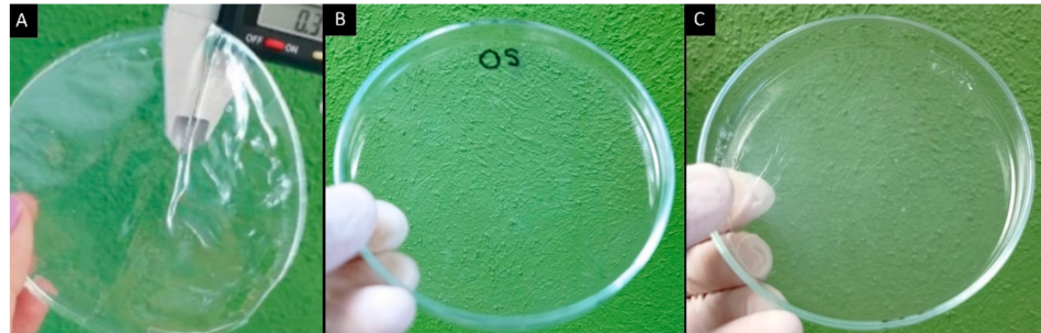
Figure 1. Developed films: (A) formulation 6 (plasticizers and OS), (B) OS without plasticizers, and (C) NS, prepared using the solution casting method.
