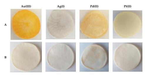
**Figure 7.** The polymer inclusion membranes containing 2,6-bis(4-methoxybenzoyl)-diaminopyridine after processes: membrane extraction (**A**), membrane back-extraction (**B**).
