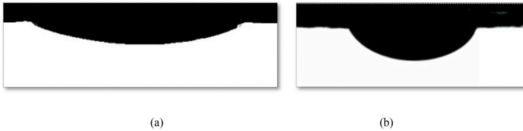
Fig. 8. Measurement of contact angle of glass. (a) Oil-wet glass before the test. (b) Glass after contact with multi-metal in optimal condition.
