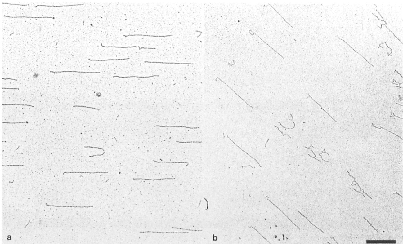
Figure 7. Electron microscopic images of mildly proteolyzed TII B and of titin prepared by the procedure of Itoh et al. (1986). a shows TII B previously mildly treated with trypsin. b shows the morphology of TII purified according to Itoh et al. (1986). In both cases the material was passed through the GPC column and oriented by centrifugation (see Materials and Methods and Fig. 5). Note that both preparations appear as headless rods with a more heterogeneous length distribution. In addition, such molecules are less well oriented than TII B (see Fig. 5). Bar, 500 nm.
