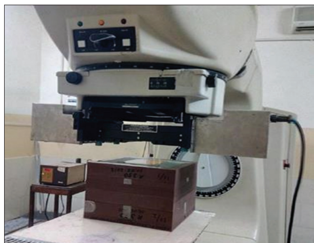
Figure 2: A typical experimental setup with prototype multileaf collimators attached to the telecobalt machine
