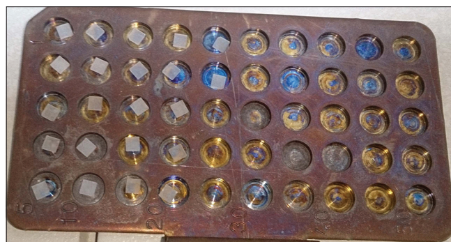
Figure 2: Thermoluminescent dosimeter Chips (LiF)
