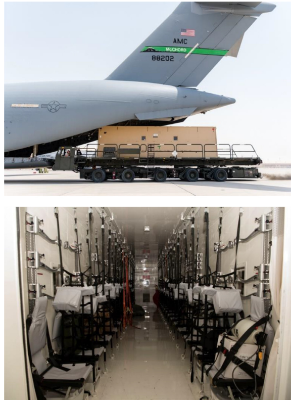
Figure 1. A Negatively Pressurized Conex. The top photograph shows a Negatively Pressurized Conex being loaded onto a C-17 Globemaster III ( https://www.af.mil/News/Article-Display/Article/2517264/negative-for-covid-19/ ). The bottom photograph shows the interior of a Negatively Pressurized Conex ( https://usdefensemilitary.com/new-kid-on-the-block-negatively-pressurized-conex-npc-arrives-at-ramstein/ ).
