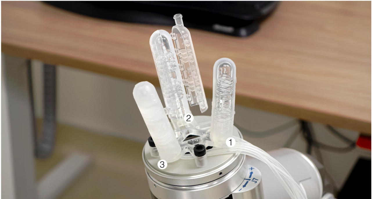
Fig 1. Negshell casting used for a three-finger soft robotic gripper. Pictured are three stages of negshell casting from the rightmost to the leftmost finger: 1. 3D-printed structural and negshell cores, 2. The cores placed in 3D-printed molds to be injected with silicone rubber, and 3. A completed finger ready to be actuated.
