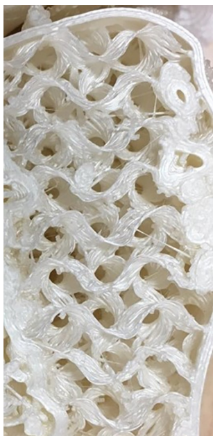
Figure 11 An example of a 3D print with an infill of 20% with gyroid structure, resembling the tactile feel of cancellous bone.
