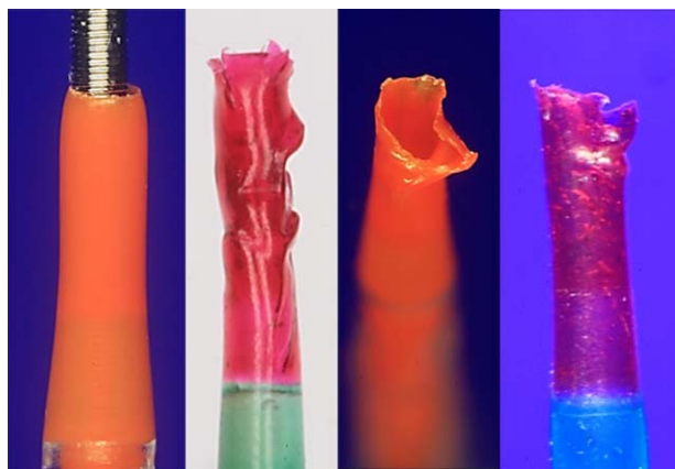
FIGURE 1 Balloon catheter tips retrieved from patients. The left most panel shows an undamaged tip. The rightward 3 panels show damaged balloon tips from 3 different manufacturers. While in these examples the flaring is marked, if of lesser degree it may not be detectable with the naked eye
