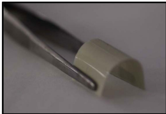
Figure 7. PDMS-micro-diamond composite thin film produced using spin coating approach.
