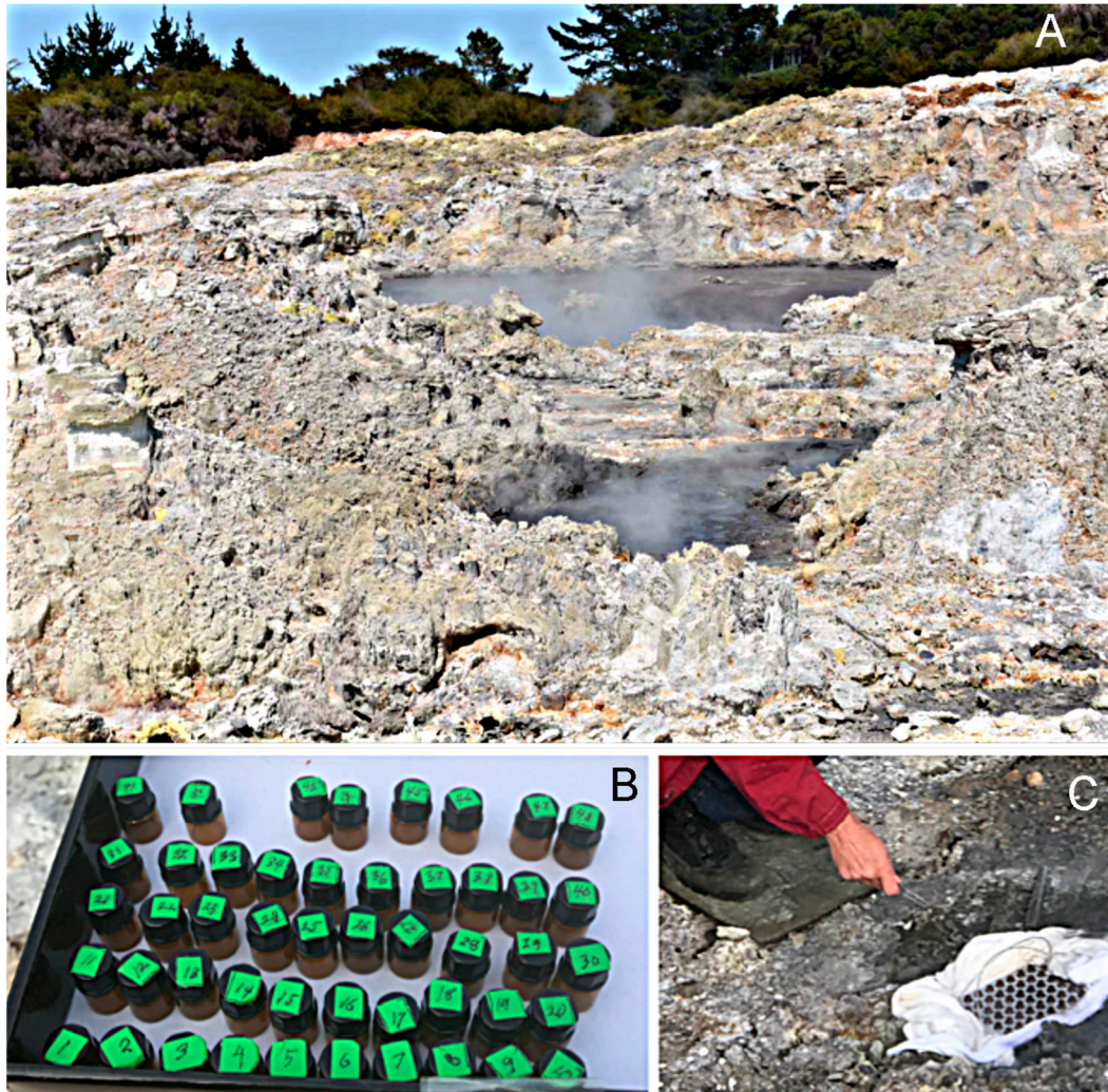
Figure 5. (A). Hell's Gate hot spring site near Rotorua, New Zealand. (B) shows vials with samples prepared beforehand, and (C) shows the vials in place in a shallow pool of water. White fabric was placed around the container to prevent boiling water splashes from falling into the samples.
