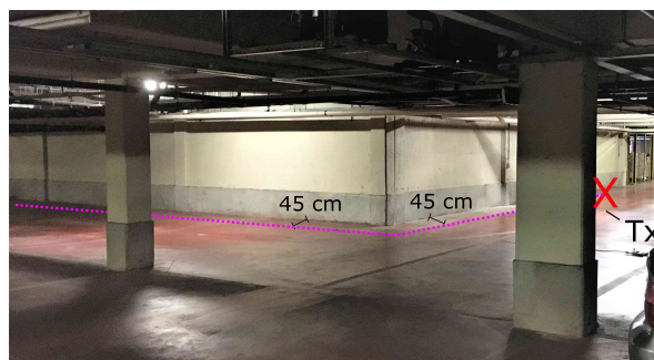
Figure 5. Scenario WOC: View of the outside corner. The Tx is indicated by the red X. The measurement path is represented by the dashed purple line. The underground parking garage was almost completely empty at the time of the measurement.
