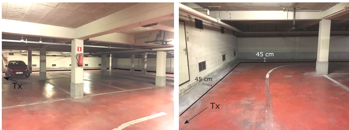
Figure 4. Scenario WIC: View showing the wall and the corner where the measurement takes place (left) and a close-up (right). The measurement path is indicated by the black line, the location of the Tx is pointed to by the arrow. The underground parking garage was almost completely empty at this time.
