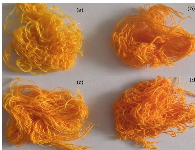
**Figure 8.** Photo of samples. (a) The blended yarns dyed with reactive yellow K-R; (b) the blended yarns dyed with reactive yellow B-4RFN; (c) the blended yarns dyed with reactive yellow K-R and fixed with DM-2158; (d) the blended yarns dyed with reactive yellow B-4RFN and fixed with DM-2158.
