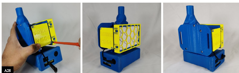
Fig. 13. Assembly instruction for step 28. A28: finish the assembly of the gear body by installing the cover with two screws. Front and back pictures of the gear body on the final assembly.
