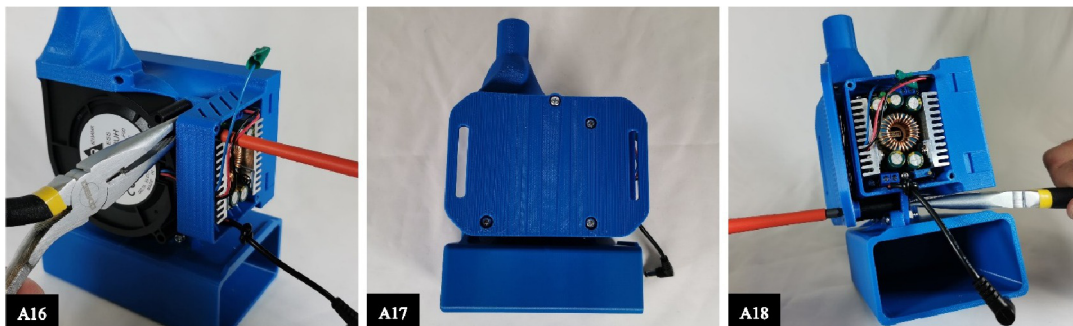
Fig. 9. Assembly instructions from steps 16 to 18. A16: tight evenly the fasteners of needed for the voltage regulator, A17: mount the belt support behind the air blower and put the fasteners in the joints, A18: install nuts on every bolt and tight all the fasteners evenly.
