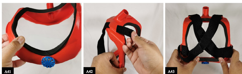
Fig. 18. Assembly instructions from steps 41 to 43. A41: confirm the neoprene band has no gaps along all the contour of the mask, A42: pass the flexible straps on the mask joints, and A43: form a cross shape with them.
