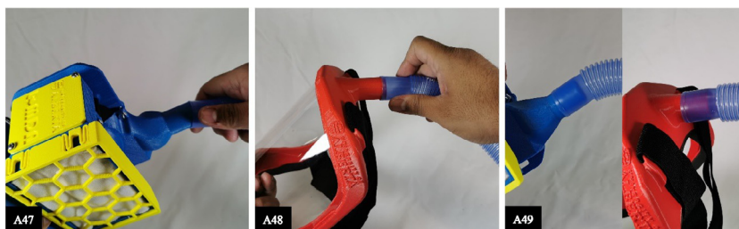
Fig. 20. Assembly instructions from steps 47 to 49. A47: insert one end of the CPAP hose on the fitting of the gear body, A48: put the other end in the mask, and A49: confirm each end of the hose cover at least 2 cm of the fitting.
