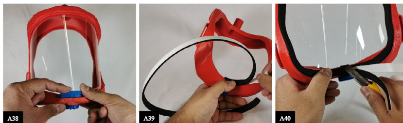
Fig. 17. Assembly instructions from steps 38 to 40. A38: secure the screen in the mask with the front lock, A39: cut a piece of neoprene tape and put in on the contour of the mask, and A40: cut the remaining of the tape once both ends are together.
