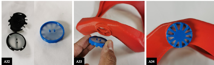
Fig. 15. Assembly instructions from steps 32 to 34. A32: take the film from the mask valve and place it on the exhaust cover, A34: locate the pins from the cover with the bottom of the mask, and A34: push the exhaust cover to fit with the bottom port.
