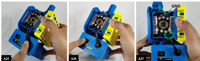
Fig. 12. Assembly instructions from steps 25 to 27. A25: connect the 12 V wire on the battery, A26: turn on the battery, and A27: regulate the output of the electric board to 6.57 V.
