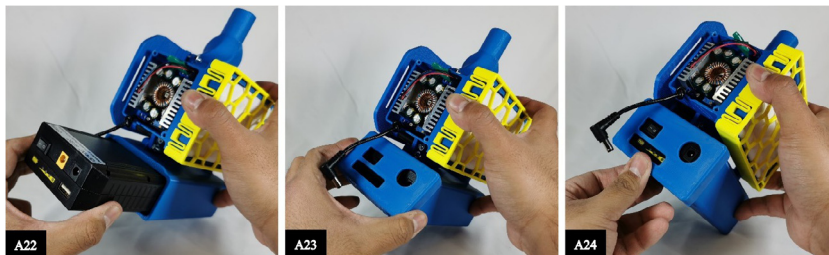
Fig. 11. Assembly instructions from steps 22 to 24. A22: Slide the battery in its holder, A23: start installing the battery cover with the top flange, and A24: finish the clamping securing the spring locks.
