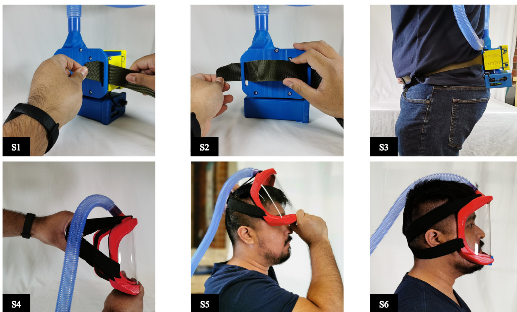
Fig. 22. Steps for correct wear of the respirator. S1: Pass the belt from the left end of the gear, S2: pass the belt thru the other end and balance the length to leave the device in the middle, S3: buckle the belt and turn on the battery, S4: grab the mask with both hand, one holding the straps and the other holding the bottom of the mask, S5: start wearing the mask by stretching the strap and pull from the back and top of your head towards the front and bottom, and S6: fit the mask to your best comfort.
