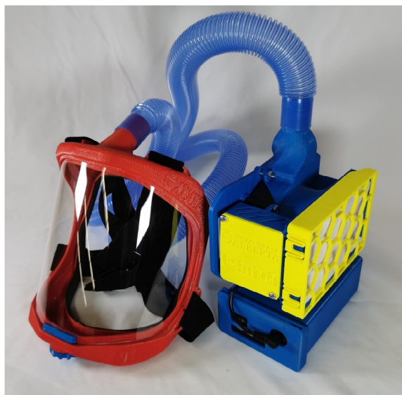
Fig. 21. Full assembly of powered and ergonomic personal respirator.
