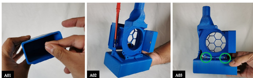
Fig. 4. Assembly instructions from steps 1 to 3. A01: insert the #8-32 nut inside the figure of the battery holder, A02: screw the vertical bolt, A03: Place two #8-32 × 3/4 bolts in the union of the battery holder and the gear body.
