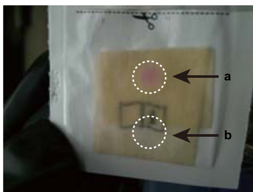
Fig. 3 Checking the oxygen level with an anaerobic indicator. The pink spot indicated by the arrow marked a shows that the oxygen level of the buffer is not sufficient for an anaerobic experiment. The sample indicated by the arrow labeled b shows that the oxygen level of the buffer is sufficient for the anaerobic experiment
