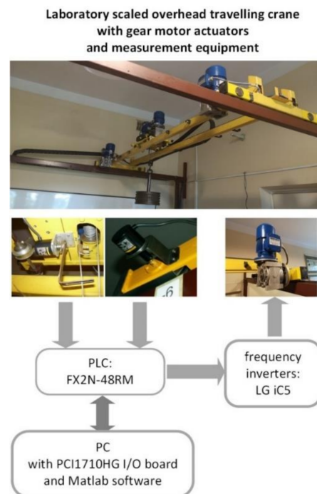
Figure 11. The laboratory stand.
