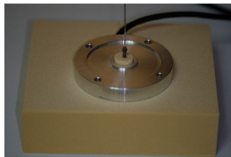
Fig. 2 A load cell was placed between 12-mm- and 20-mm-thick Sawbone blocks (grade 15 pcf, [0.24 g/cm 3 ]), which maintained a 1-mm space between the blocks. After placing the guide pin into the center of the block, drilling was performed to a predetermined depth, and the screws were inserted
