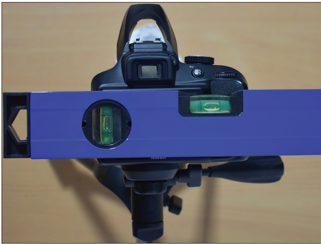
Figure 1: Digital camera with leveling bubble in place
