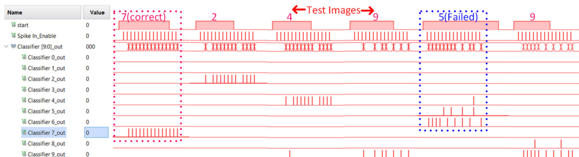
Figure 12. The measurement results for Digital SNN showing the correct classification of different input images along with the failed classification of input image '5'.
