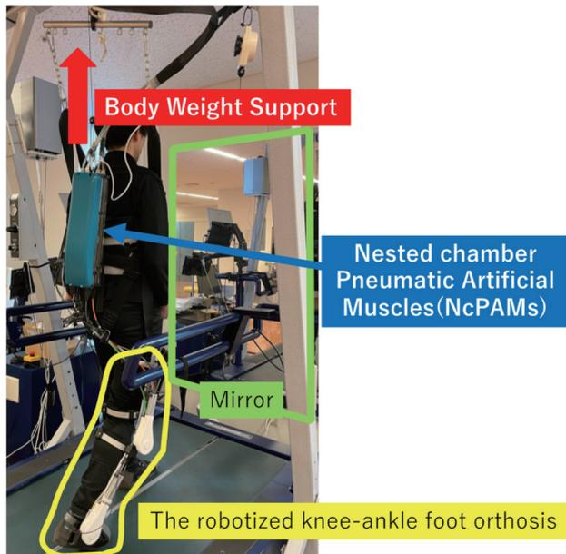
**Fig. 2.** Robotized knee–ankle–foot orthosis.
