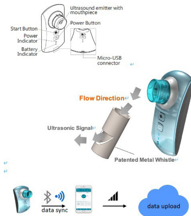
Figure 1 The Restart system's architecture which including a remote spirometry, a mobile phone and App.
