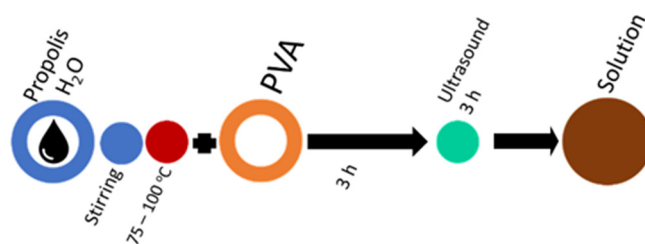
Figure 6. Solution mixing sequence for propolis water integration into electrospinning solution.
