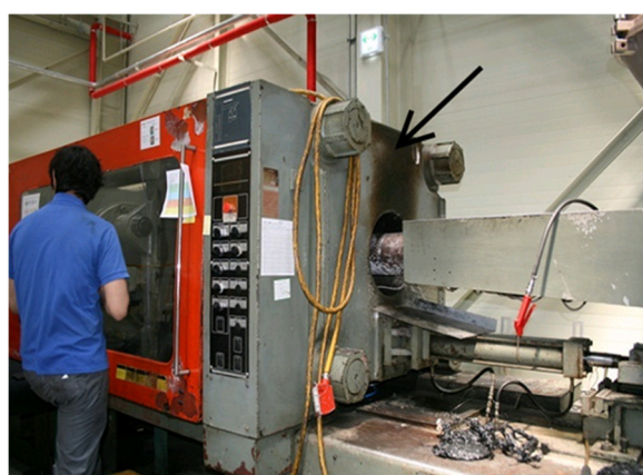
Figure 2 Injection port of the plastic resins (pouring resins into the hopper of the molding machine). The arrow indicates discoloration caused by hume leakage when injection processing or changing the raw material.
