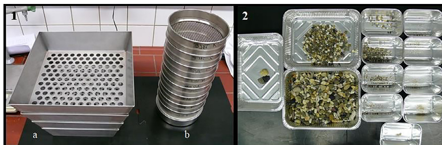
Figure 4. Fractionation of the gastro- and enterolith mixtures by means of a shaking box (1a) and a sieve tower (1b); gastroliths from the contents of a gizzard (2) divided into 12 fractions.
