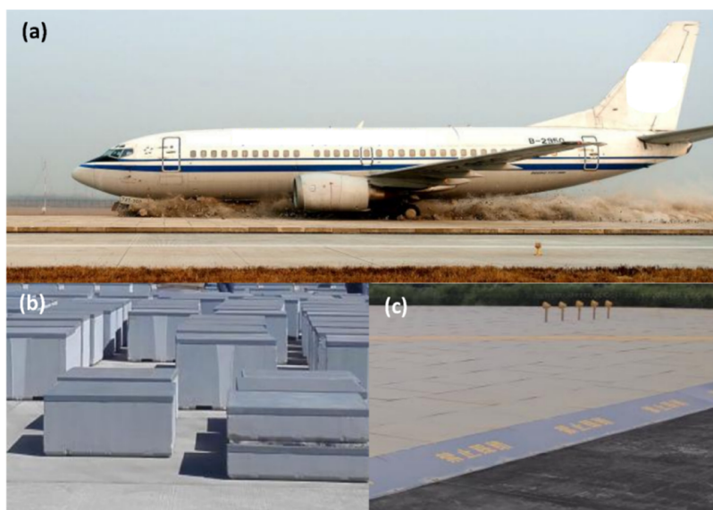
Figure 1. (a) Snapshot of a field test of EMAS arresting a Boeing 737 airplane in Tianjin Binhai Int. Airport by Civil Aviation Administration of China (CAAC). (b) SFCF blocks of EMAS unit ready for installation. (c) Picture of EMAS installed in the Nyingchi Mainling Airport, Tibet, China (photograph courtesy of Y.Z. Copyright 2022).
