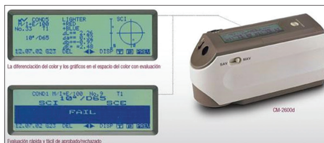
Figure 2: Illustration of the spectrophotometer used in research and industry (Konica Minolta CM-2600d) (Source: http://www.quiminet.com )
