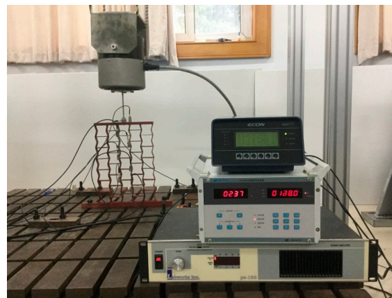
Figure 13. Frequency response experiment of the auxetic honeycombs.
