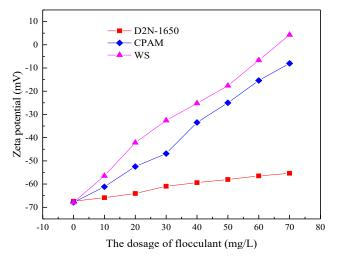
Figure 6. The effect of flocculant on Zeta potential.
