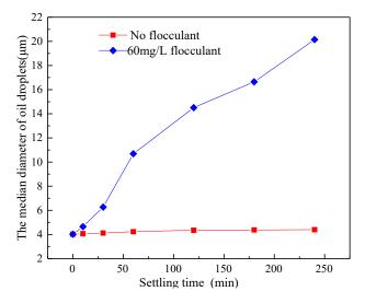
Figure 7. The effect of flocculant on the median diameter of oil droplets.
