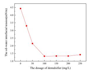
Figure 1. The effect of demulsifier on interfacial tension.
