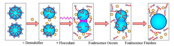
Figure 9. Demulsification-Flocculation mechanism.
