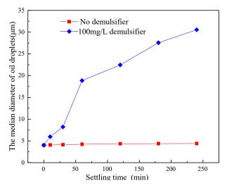
Figure 3. The effect of demulsifier on the median diameter of oil droplets.
