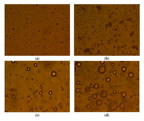
**Figure 4.** The effect of demulsifier on the size of oil droplets. (**a**) Settlement without demulsifier for 0 min, (**b**) settlement without demulsifier for 120 min, (**c**) settlement with demulsifier for 0 min, (**d**) settlement with demulsifier for 120 min.
