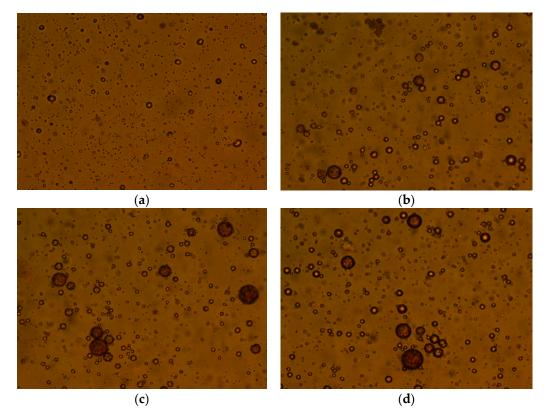
**Figure 8.** The effect of flocculant on the size of oil droplet. (**a**) Settlement without flocculant for 0 min, (**b**) settlement without flocculant for 120 min, (**c**) settlement with flocculant for 0 min, (**d**) settlement with flocculant for 120 min.
