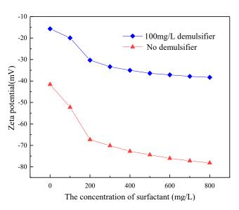
Figure 2. The effect of demulsifier on Zeta potential.
