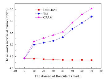
Figure 5. The effect of flocculant on interfacial tension.
