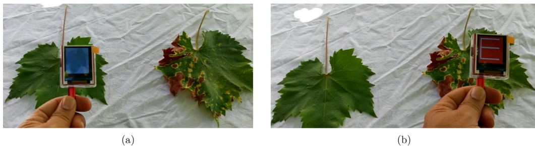
Fig. 2. OpenMV Cam with LCD display that shows the classification response applied to Esca disease (CNN trained on ESCA-dataset). (a) Healthy leaf (no tag), (b) Leaf affected by Esca disease correctly detected as shown in the LCD display (tag 'E').
