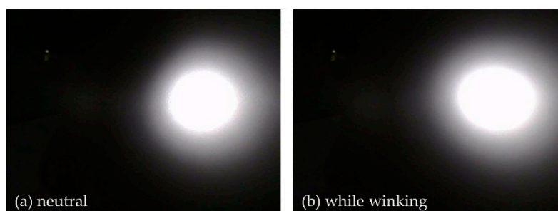
Figure 4. Images of IR laterally propagated through the skin: (a) IR SRDR image captured with no facial gesture and (b) captured IR SRDR image during a wink gesture by the user. The brightness of the white region in these images represents the intensity of the IR SRDR.
